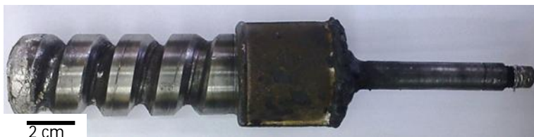
Fig.1 Steel screw used for melt shearing process.
